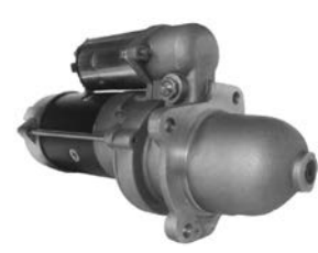
110590 Starter 12 V, 2.8 kW Replacing: LNS2830 Servicing: Bobcat, Perkins B+ M10, Total length 339.00, Gear type GR, Clutch type Dry, Mount. holes 3 (0), Waterproof Replaces: 22MT, 27MT, 28MT. A: 88.90 B: 46.00 mm
