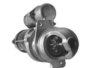
110602 Starter 12 V, 2.8 kW Replacing: LNS2820 Servicing: Bobcat, Clark, Perkins B+ M10, Total length 339.00, Gear type GR, Clutch type Dry, Mount. holes 3 (0), Oil sealed Replacing: 22MT, 28MT. A: 89.00 B: 46.00 mm
