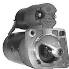
111025 Starter 12 V, 0.8 kW Replacing: R80K, R80.04 Servicing: Autobianchi, Fiat, Lancia B+ M8, Total length 199.25, Gear type DD, Mount. holes 3 (2) A: 64.00 B: 11.00 mm
