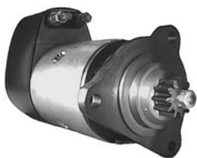
110582 Starter 24 V, 5.4 kW Replacing: R23.06, 6060000 Servicing: Iveco B+ M10, B- M10, Total length 384.00, Gear type DD, Mount. holes 3 (0) A: 92.00 B: 47.00 mm
