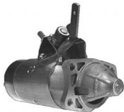
110608 Starter 12 V, 0.5 kW Replacing: B76-0.5/12 Servicing: Fiat B+ M8, Total length 233.75, Gear type DD, Clutch type Dry, Mount. holes 3 (0) A: 61.90 B: 7.70 mm
