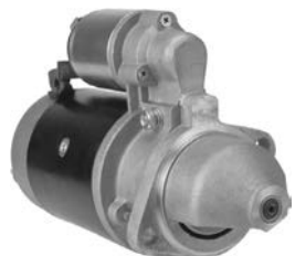
114265 Starter 12 V, 2.7 kW Replacing: 0001366009, 0001354099 Servicing: VM Motori B+ M10, Total length 295.00, Mount. holes 2 (0) A: 82.50 B: 21.50 mm
