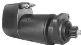
110932 Starter 24 V, 5.4 kW Replacing: R23.24 Servicing: DAF B+ M10, B- M10, Total length 384.50, Gear type DD, Mount. holes 3 (0), Insulated return A: 88.85 B: 47.00 mm
