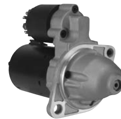
114297 Starter 12 V, 1.2 kW Replacing: 0001107426, 0001107425 Servicing: BMW B+ M8, Total length 199.00, Gear type DD/GR, Mount. holes 2 (1) A: 76.00 B: 25.00 mm
