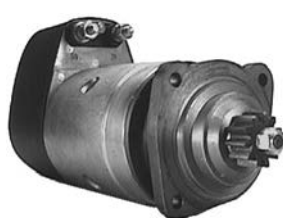
111046 Starter 24 V, 6.6 kW Replacing: R22.06, 0060000 Servicing: MAN, Volvo B+ M10, Total length 404.00, Gear type DD, Mount. holes 3 (0) A: 88.85 B: 48.00 mm
