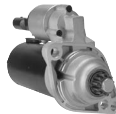
114299 Starter 12 V, 1.7 kW Replacing: 0001123029, 0001123028 Servicing: Audi, Seat, Skoda, VW B+ M8, 15a Plug, Total length 232.00, Gear type GR, Mount. holes 3 (0) A: 76.20 B: 56.00 mm
