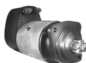
111249 Starter 24 V, 5.4 kW Replacing: R23.14, 6140000 Servicing: Various Industrial applications B+ M10, Total length 381.80, Gear type DD, Mount. holes 3 (0), Waterproof A: 89.00 B: 48.25 mm
