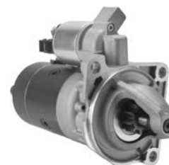
114304 Starter 12 V, 2.3 kW Replacing: 6033AB1J00, 0001218822 Servicing: VW B+ M8, Total length 272.00, Gear type GR, Clutch type Dry, Mount. holes 3 (0) A: 110.00 B: 27.00 mm
