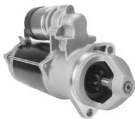
114220 Starter 24 V, 4.0 kW Replacing: 0001231018, 0001101110 Servicing: Deutz-Fahr B+ M10, Total length 315.00, Gear type GR, Mount. holes 2 (0) A: 82.50 B: 25.00 mm
