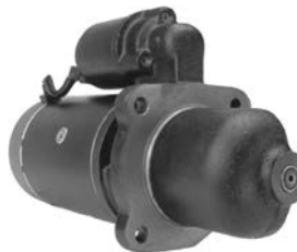
110527 Starter 24 V, 4.0 kW Replacing: LNS4524/13, 859535, 857472 Servicing: Scania, Steyr B+ M10, Total length 342.00, Gear type DD, Mount. holes 3 (0) A: 89.00 B: 46.50 mm
