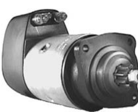
110538 Starter 12 V, 3.6 kW Replacing: 860542 Servicing: Volvo Penta B+ M10, B- M10, Total length 384.00, Gear type DD, Mount. holes 3 (0), Insulated return A: 89.00 B: 47.00 mm
