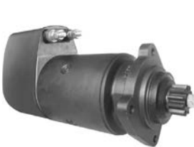
110535 Starter 24 V, 5.4 kW Replacing: 860655, 860115 Servicing: Iveco B+ M10, B- M10, Total length 384.00, Gear type DD, Mount. holes 3 (0) A: 89.00 B: 47.00 mm
