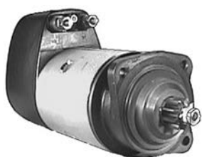
110601 Starter 24 V, 5.4 kW Replacing: R23.13, 6130000 Servicing: Mercedes-Benz, Steyr B+ M10, Total length 384.25, Gear type DD, Mount. holes 3 (0) A: 88.85 B: 47.50 mm
