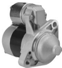
114199 Starter 12 V, 0.7 kW Replacing: 0001116008 Servicing: Nissan B+ M8x1.25, Total length 166.00, Gear type DD, Mount. holes 2 (1) A: 70.00 B: 11.00 mm
