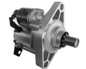
113392 Starter 12 V, 1.6 kW Replacing: SM442-29, SM442-01 Servicing: Acura, Honda B+ M8, Total length 210.00, Gear type GR, Mount. holes 2 (0) A: 74.90 B: 33.00 mm
