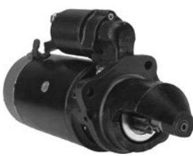
110525 Starter 12 V, 3.0 kW Replacing: 860130, 860109 Servicing: Claas, Mercedes-Benz B+ M10, Total length 341.00, Gear type DD, Mount. holes 3 (0) A: 89.00 B: 48.00 mm
