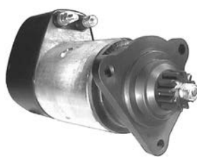
110980 Starter 24 V, 5.4 kW Replacing: R23.34, 6340000 Servicing: Volvo B+ M10, B- M10, Total length 387.00, Gear type DD, Mount. holes 3 (0) A: 92.00 B: 47.00 mm
