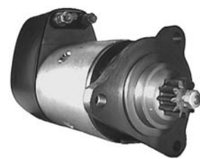
110582 Starter 24 V, 5.4 kW Replacing: 860516, 860125 Servicing: Iveco B+ M10, B- M10, Total length 384.00, Gear type DD, Mount. holes 3 (0) A: 92.00 B: 47.00 mm
