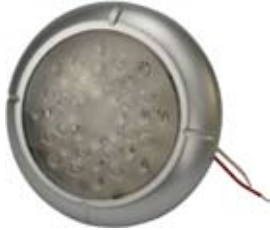
171678 LED Interior Lamp 12 / 24 V., Dimension 140 x 29, Mount. holes dist. 123, E-Approval CE, IP66.
