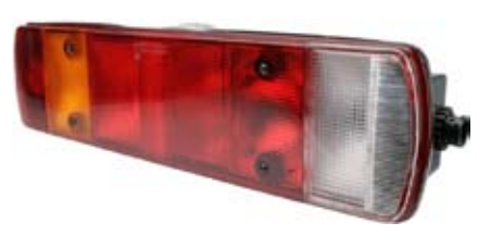
171320 Multi Function Lamp Servicing: Volvo. Dimension 516 x 130 x 80, Mount. holes dist. 160, Socket BA15s, E-Approval Yes, 2 Bulb Holders for Tail Light. Lens: Cargo 171322. See Survey.
