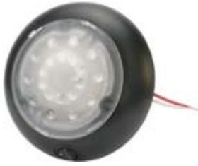
171677 LED Interior Lamp 12 / 24 V., 1.5 Watt, Mount. holes dist. 75, E-Approval E11 10R-024557, With switch
