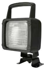
170983 Work Lamp Model COMPACT 3000, Type H3, Colour Black, Light aperture 73 x 73, Tightness norm IP 65, External plug for 6.30mm flat plug connection.
