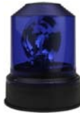
171017 Rotating Beacon 12 / 24 V., Colour Blue, O.D. 145, H. 192, Lens PMMA/ACRYL, Bulb H1, Tightness norm IP 55, Approval E3 020157,
