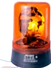
171705 Rotating Beacon 12 / 24 V., Colour Orange, O.D. 160, H. 220, Lens PMMA/ACRYL, Bulb H1, Approval E2 0089004, Lens: Cargo 170308. Motor: Cargo 170505,170506.
