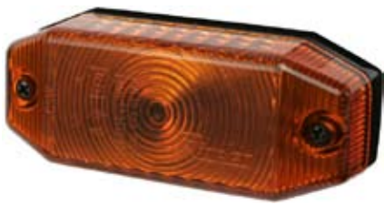
171369 Side Marker Lamp Dimension 102 x 42 x 28, Mount. holes dist. 65, E-Approval Yes,
