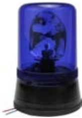
170798 Rotating Beacon 12 / 24 V., Colour Blue, O.D. 160, H. 220, Lens PMMA/ACRYL, Bulb H1, Approval E2 0089004, Lens: Cargo 170366. Motor: Cargo 170505, 170506.
