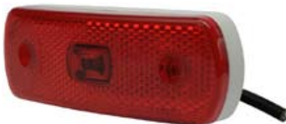
171579 LED Tail Lamp 12 V., Dimension 104 x 36 x 19.6, Mount. holes dist. 70, E-Approval Yes,
