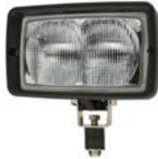
171167 Work Lamp 12/24/36/48 V., Type H3, Colour Black, Light aperture 136 x 88, Tightness norm IP 54,
