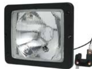
170867 Head Lamp 12 - 24 V., Dimension 172 x 144 x 89, Socket BA9s, E-Approval Yes, Heat Resistant plastic reflector bonded w/ glass lens. Flush fitting head lamp. Build-in depth: 69.00mm.
