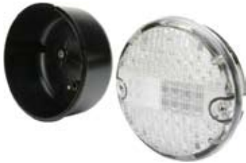
171684 Reversing Lamp LED 9-33 V., Dimension 140 x 80, Mount. holes dist. 45, E-Approval Yes, Can be flush mounted by using 171266
