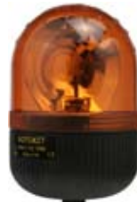
171351 Rotating Beacon 24 V., Colour Orange, O.D. 114, H. 167, Lens Polycarbonat, Bulb H1, Tightness norm IP 44, Approval E9 004021, Fixing bases: Cargo: 171348, 171349, 171352, 171353, 171354, 171355.
