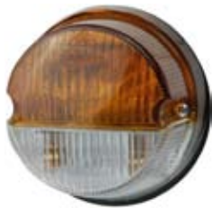
171215 Flasher/Position Lamp Dimension 80 x 43, Mount. holes dist. 45, E-Approval Yes, Lens: Cargo 171248.
