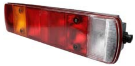
171318 Multi Function Lamp Servicing: Volvo. Dimension 516 x 130 x 80, Mount. holes dist. 160, Socket BA15s, E-Approval Yes, 2 Bulb Holders for Tail Light. Lens: Cargo 171322. See Survey.
