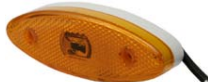
171607 LED Side Marker Lamp 24 V., Dimension 114 x 39 x 18.5, Mount. holes dist. 70, E-Approval Yes,
