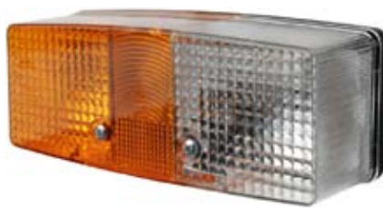
171218 Flasher/Position Lamp Dimension 158 x 64 x 51, Mount. holes dist. 98/45, E-Approval E12 7100, Lens: Cargo 171261.
