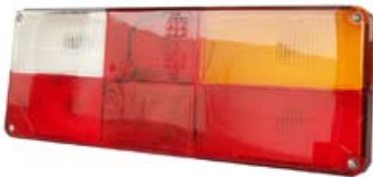
171287# Multi Function Lamp Servicing: Iveco Eurotech. Dimension 378 x 145 x 82, Mount. holes dist. 326, Socket BA10s, 2 Bulb Holders for Tail Light. Lens: Cargo 171293. See Survey.
