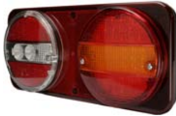
171665 LED Multi Function Lamp 12 / 24 V., Dimension 336 x 151 x 67, Mount. holes dist. 152, E-Approval Yes, See Survey.
