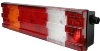
171311 Multi Function Lamp Servicing: Mercedes Actros. Dimension 525 x 139 x 83, Mount. holes dist. 200, Socket BA15s, E-Approval Yes, Optional use. Lens: Cargo 171521. See Survey.
