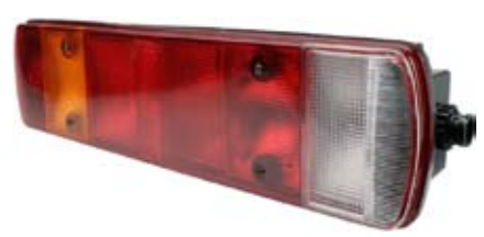
171321 Multi Function Lamp Servicing: Volvo. Dimension 516 x 130 x 80, Mount. holes dist. 160, Socket BA15s, E-Approval Yes, 2 Bulb Holders for Tail Light. Lens: Cargo 171322. See Survey.
