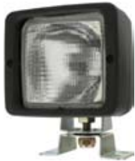
170982 Work Lamp Type H3, Colour Black, Light aperture 73 x 73, External plug for 6.30mm flat plug connection.
