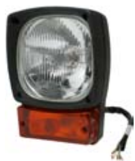
170926 Head Lamp 24 V., Dimension 155 x 208 x 128, E-Approval E2 02907029/E5 01626, Lens: Cargo 171007.
