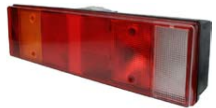
171297 Multi Function Lamp Servicing: DAF. Dimension 465 x 130 x 83, Mount. holes dist. 152, Socket BA15s, E-Approval Yes, 2 Bulb Holders for Tail Light. Lens: Cargo 170968. See Survey.
