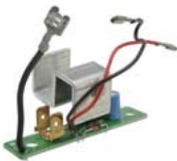
170527 Converter Servicing: Cargo 170491, 171018. 12 / 24 V.
