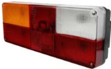
171288# Multi Function Lamp Servicing: Iveco Eurotech. Dimension 378 x 145 x 82, Mount. holes dist. 326, Socket BA10s, 2 Bulb Holders for Tail Light. Lens: Cargo 171294. See Survey.
