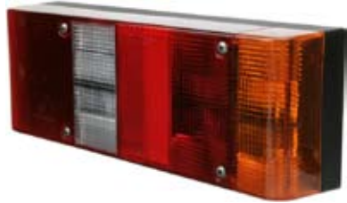
171210 Multi Function Lamp Dimension 281 x 99 x 56, Mount. holes dist. 184, Socket BA15s, See Survey.
