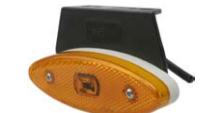
171608 LED Side Marker Lamp 24 V., Dimension 114 x 39 x 18.5, Mount. holes dist. 52, E-Approval Yes,
