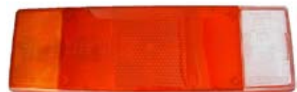
170665 Lens, Rear Lamp Servicing: Cargo 170603, 170602, 171585, 170586
