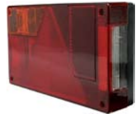
171054 Multi Function Lamp Dimension 235 x 135 x 52, Mount. holes dist. 152, Socket S8.5, E-Approval E3 56117, Lens: Cargo 171057. Plug: Cargo 171372, 171373. See Survey.
