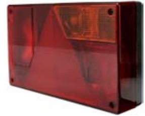
171053 Multi Function Lamp Dimension 235 x 135 x 52, Mount. holes dist. 152, Socket S8.5, Lens: Cargo 171056. See Survey.
