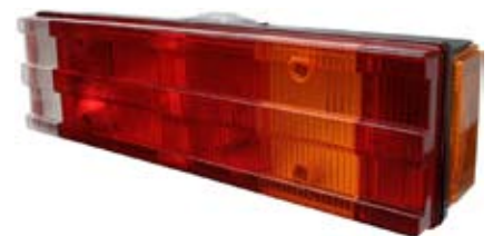
171302 Multi Function Lamp Servicing: Mercedes Atego. Dimension 465 x 130 x 90, Mount. holes dist. 152, Socket BA15s, E-Approval Yes, Optional use. 2 Bulb Holders for Tail Light. Lens: Cargo 171307. See Survey.
