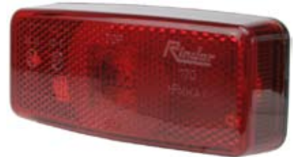
170886 Tail Lamp Dimension 110 x 46 x 26, Mount. holes dist. 85, E-Approval E4 9337, Lens: Cargo 171334.
