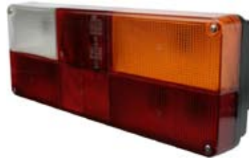
171290# Multi Function Lamp Servicing: Iveco Turbo Star. Dimension 378 x 145 x 82, Mount. holes dist. 326, 2 Bulb Holders for Tail Light. Lens: Cargo 171293. See Survey.
