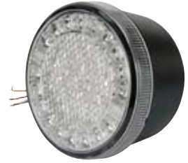
171725 LED Tail-Position Lamp 12 / 24 V., Dimension 122 x 84.5, Mount. holes dist. 44, E-Approval Yes, Ring=amber, center=red
