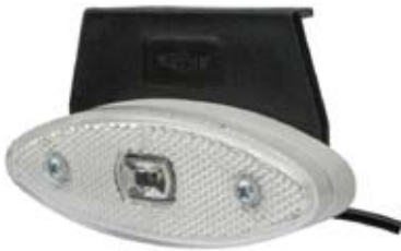
171610 LED Position Lamp 24 V., Dimension 114 x 39 x 18.5, Mount. holes dist. 52, E-Approval Yes,
