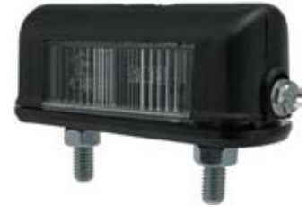
171224 Number Plate Lamp 12 / 24 V., 5 Watt, Dimension 82 x 26 x 31, Mount. holes dist. 45, E-Approval E12 4033,
