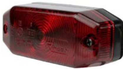
171331 Tail Lamp Dimension 102 x 42 x 28, Mount. holes dist. 65, E-Approval E9 01490,
