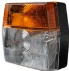
171216 Flasher/Position Lamp Dimension 93 x 99 x 50, Mount. holes dist. 45, E-Approval E12 6078, Lens: Cargo 171254.
