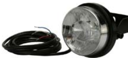
171699 LED Daytime Running Light 12 / 24 V., 2.5 / 2.6 Watt, Dimension 93 x 89 x 69, Mount. holes dist. 45, E-Approval 000877,
