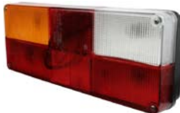
171292# Multi Function Lamp Servicing: Iveco Turbo Star. Dimension 378 x 145 x 82, Mount. holes dist. 326, Socket BA15s, 2 Bulb Holders for Tail Light. Lens: Cargo 171294. See Survey.
