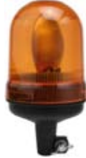
170971 Rotating Beacon 12 V., Colour Orange, O.D. 142, H. 235.5, Lens Polycarbonat, Bulb H1, Approval E3 00a151160, Lens: Cargo 171463.
