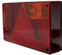
171051 Multi Function Lamp Dimension 235 x 135 x 52, Mount. holes dist. 152, Socket S8.5, E-Approval E3 56117, Lens: Cargo 171056. Plug: Cargo 171372, 171373. See Survey.
