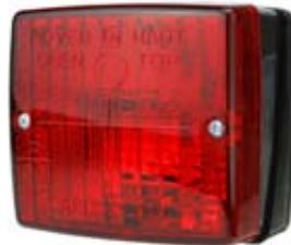
170928 Rear Fog Lamp Dimension 102 x 95 x 55, Mount. holes dist. 77, E-Approval E6 8703,
