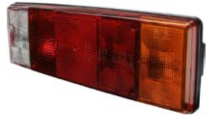
170602 Multi Function Lamp Servicing: RVI Renault, Pegaso Dimension 406 x 135 x 74, Mount. holes dist. 152, Socket BA15s, E-Approval Yes, Lens: Cargo 170665. See Survey.
