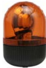
171350 Rotating Beacon 12 V., Colour Orange, O.D. 114, H. 167, Lens Polycarbonat, Bulb H1, Tightness norm IP 44, Approval E9 004021, Fixing bases: Cargo: 171348, 171349, 171352, 171353, 171354, 171355.
