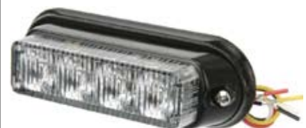
171644 LED Flash 12 / 24 V., Colour Blue, H. 29, Bulb LED, Approval 033959, 12 Flash patterns. Multi-module synchronization. Bracket: Cargo 171657.
