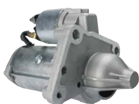
113933 Starter 12 V, 1.5 kW Replacing: TS18E13, D7G3, 190895 Servicing: Citroen, Mini, Peugeot, Toyota B+ M8, Total length 220.00, Gear type GR, Mounting holes 4 (2) B: 13.00 mm
