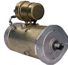
112138# DC Motor 12 V, 0.8 kW Replacing: AME1706, AME1609, 11.212.192, 11.212.147, 47045933, 47045911, 47045811, 19024716, 19024699, 19024698 OD 78.00, Total length 184.00, Pulley w/o, Rpm./ max. 2700
