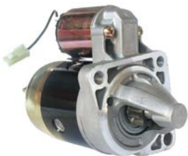
110149 Starter 12 V, 0.9 kW Replacing: M38382, 1EM0088 Servicing: Mazda, Mercury B+ M8, Total length 198.00, Gear type DD, Mounting holes 3 (2) A: 74.00 B: 15.00 mm
