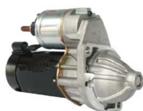
111931 Starter 12 V, 1.1 kW Replacing: D7E8, D7E4, D7E38, D7E18, D6RAP229, D6RA83, D6G5 Servicing: Mercedes-Benz B+ M8, Total length 212.00, Gear type GR, Mounting holes 2 (0) A: 70.00 B: 15.00 mm
