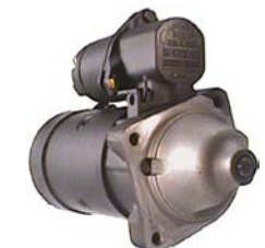
110338 Starter 12 V, 0.8 kW Replacing: 9141325 Servicing: Fiat, Lancia, Zastava B+ M8, Total length 254.00, Gear type DD, Mounting holes 3 (3) A: 66.90 B: 12.00 mm
