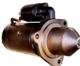
112055 Starter 24 V, 5.2 kW Replacing: 860304 Servicing: DAF B+ M10, Total length 340.00, Gear type DD, Mounting holes 3 (0) A: 110.00 B: 48.00 mm
