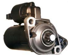
111909 Starter 12 V, 1.1 kW Replacing: D7E55, D7E51, 190396 Servicing: Audi, Ford, Seat, Skoda, VW B+ M8, Total length 212.00, Gear type GR, Mounting holes 3 (0) A: 76.25 B: 32.00 mm
