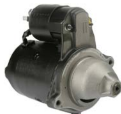
111066 Starter 12 V, 1.05 kW Replacing: 6242, 6240, 618795, 618565, 618078, 618077, 534050, 534046, 453016 Servicing: Citroen, Fiat, Peugeot, Talbot B+ M8, Total length 197.00, Gear type DD, Mounting holes 2 (2) A: 65.90 B: 22.00 mm
