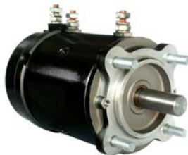
112577 DC Motor 12 V, 1.8 kW Replacing: MBJ6304, MBJ6202, MBJ6201, MBJ4407, MBJ4402, MBJ4209, MBJ4202, MBJ4201, 46-4157 OD 113.30, Total length 211.00, Pulley w/o, Rpm./ max. 2600 Shaft 19.00 mm.thread on thru bolts: 3/8 unF x 22.50.
