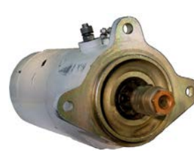
112084 Starter 12 V, 3.6 kW Replacing: 870645 Servicing: Ford B+ M8, 15a M5, Total length 370.50, Gear type DD, Mounting holes 3 (0), Insulated return, Oil sealed A: 92.10 B: 20.60 mm
