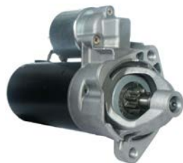
111694 Starter 12 V, 1.8 kW Replacing: D7R33 Servicing: Audi, Ferrari, Seat, Skoda, VW B+ M8, Total length 270.00, Gear type GR, Mounting holes 2 (2) A: 82.00 B: 16.00 mm
