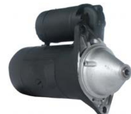
110364 Starter 12 V, 0.65 kW Replacing: D9E128 Servicing: Opel, Vauxhall B+ M8, 15a 6.30, Total length 229.50, Gear type DD, Mounting holes 2 (0) A: 68.00 B: 14.00 mm
