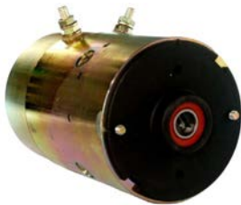
112572 # DC Motor 24 V, 1.9 kW Replacing: 0136602009, AMJ4603, 11.212.106 OD 112.00, Total length 197.00, Pulley w/o, Rpm./ max. 4300
