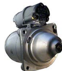
111106 Starter 12 V, 1.0 kW Replacing: 534028, 534027 Servicing: Fiat, Lancia, Seat B+ M8, Total length 232.00, Gear type DD, Mounting holes 3 (3) A: 82.00 B: 22.40 mm
