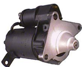
110860# Starter 12 V, 0.9 kW Replacing: 532004, 532003 Servicing: Citroen, Peugeot, Renault B+ M8, Total length 253.00, Gear type DD, Mounting holes 3 (0) A: 80.00 B: -6.00 mm
