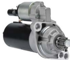
114173 Starter 12 V, 1.7 kW Replacing: 0001123021, 0001123020 Servicing: VW B+ M8, Total length 244.00, Gear type GR, Mounting holes 2 (0) A: 76.00 B: 58.00 mm
