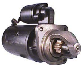
111399 Starter 24 V, 4.5 kW Replacing: LNS4524/9, 859506, 859022 Servicing: DAF B+ M10, Total length 352.50, Clutch type Wet, Gear type DD, Mounting holes 3 (0) A: 89.00 B: 38.00 mm
