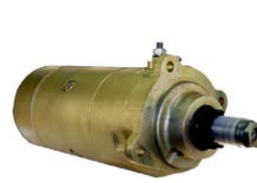
112091 Starter 24 V, 5.2 kW Replacing: 870658, 870649 Servicing: Perkins B+ M8, 15a M5, Total length 371.55, Gear type DD, Mounting holes 3 (0), Insulated return, Oil sealed A: 89.00 B: 47.00 mm
