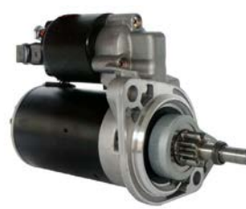
111748 Starter 12 V, 1.1 kW Replacing: 35259250 Servicing: Audi, Ford, Seat, Skoda, VW B+ M8, Total length 223.00, Gear type GR, Mounting holes 2 (0) Bushing D.E. (clutch house): Cargo 140018. A: 76.00 B: 33.00 mm
