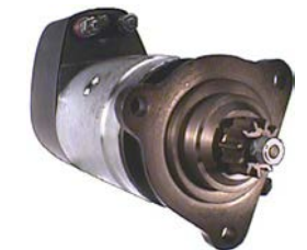
110212 Starter 24 V, 6.6 kW Replacing: 9125460, 9125130 Servicing: Iveco, Scania B+ M12, B- M10, Total length 407.00, Gear type DD, Mounting holes 3 (0) A: 92.00 B: 47.65 mm
