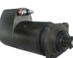
110208 Starter 24 V, 5.4 kW Replacing: 9125250 Servicing: Fiat-Allis, Mercedes-Benz, Steyr, Volvo B+ M12, B- M10, Total length 387.00, Gear type DD, Mounting holes 3 (0), Waterproof A: 89.00 B: 48.50 mm
