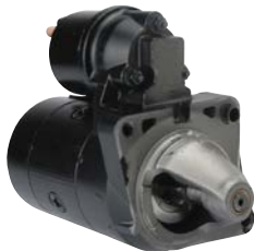
114123 Starter 12 V, 0.8 kW Replacing: F000AL0310, F000AL0309 Servicing: Fiat B+ M8, 30h M6, Total length 190.00, Gear type DD/GR, Mounting holes 3 (2) A: 64.00 B: 12.00 mm
