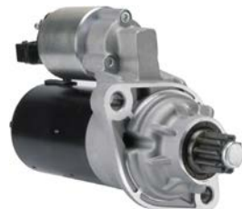
114174 Starter 12 V, 1.1 kW Replacing: 0001121023, 0001121022 Servicing: Audi, Seat, Skoda, VW B+ M8, Total length 233.90, Gear type GR, Mounting holes 2 (0) A: 76.00 B: 62.00 mm
