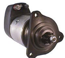
110206 Starter 24 V, 5.4 kW Replacing: 9125330, 9125260, 9125220 Servicing: Claas, Fiat-Allis, Kässbohrer, MAN, Mercedes-Benz, Neoplan, Setra B+ M12, B- M10, Total length 390.00, Gear type DD, Mounting holes 3 (0) A: 92.00 B: 47.50 mm
