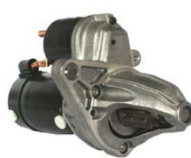
112476 Starter 12 V, 1.0 kW Replacing: D6RA811, D6RA81, D6RA181 Servicing: Honda B+ M8, Total length 229.00, Clutch type Wet, Gear type GR, Mounting holes 2 (0) A: 75.00 B: 39.00 mm
