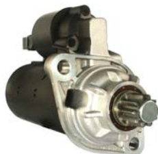
112429 Starter 12 V, 2.0 kW Replacing: D7RS50, D7RS150 Servicing: Audi, Ford, Seat, Skoda, VW B+ M8, Total length 259.00, Gear type GR, Mounting holes 2 (0) A: 76.00 B: 62.00 mm
