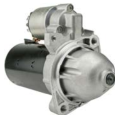
112440 Starter 12 V, 2.2 kW Replacing: D9R149, D7RP123, D7R281 Servicing: Mercedes-Benz B+ M8, Total length 240.00, Gear type GR, Mounting holes 2 (2) A: 82.50 B: 26.00 mm
