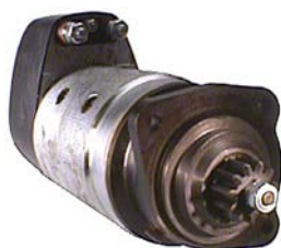
110205 Starter 24 V, 6.5 kW Replacing: D13E101TE, D13E101 Servicing: Volvo B+ M12, Total length 407.00, Gear type DD, Mounting holes 3 (0), Waterproof A: 89.00 B: 47.50 mm
