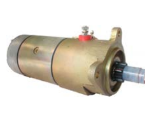
112090 Starter 24 V, 5.2 kW Replacing: 870653 Servicing: Ford B+ M8, 15a M5, Total length 371.50, Gear type DD, Mounting holes 3 (0), Insulated return, Oil sealed A: 92.00 B: 20.50 mm
