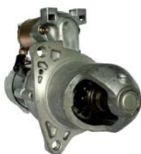
112342 Starter 24 V, 5.5 kW Replacing: MG255301, M34466, M000A0271 Servicing: Hyundai, Mitsubishi B+ M10, Total length 368.00, Gear type GR, Mounting holes 3 (0) A: 100.00 B: 68.00 mm
