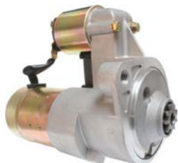
111534 Starter 12 V, 1.4 kW Replacing: 20500974 Servicing: Opel, Vauxhall B+ M8, Total length 188.00, Gear type GR, Mounting holes 2 (1) A: 77.90 B: 19.00 mm
