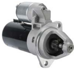
114106 Starter 12 V, 1.6 kW Replacing: 0001109043, 0001109008 Servicing: Hatz B+ M8, Total length 263.00, Mounting holes 2 (0) A: 82.50 B: 40.00 mm
