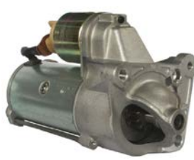
112474 Starter 12 V, 1.8 kW Replacing: D7R49, D7R48, D7R47, D7R44 Servicing: Nissan, Opel, Renault, Vauxhall, Volvo B+ M8, Total length 238.00, Clutch type Wet, Gear type GR, Mounting holes 3 (2) B: -2.00 mm
