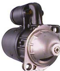
110341 Starter 12 V, 0.8 kW Replacing: D9E124 Servicing: Bedford, Opel, Vauxhall B+ M8, 15a 6.30, Total length 260.00, Gear type DD, Mounting holes 2 (0) A: 77.85 B: 15.00 mm
