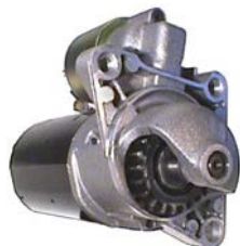
111680 Starter 12 V, 1.1 kW Replacing: PBNS1165, 20510165 Servicing: Ford B+ M8, Total length 211.75, Gear type GR, Mounting holes 3 (2) A: 71.00 B: 15.00 mm
