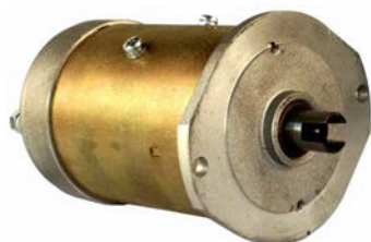
112484 # DC Motor 24 V, 0.4 kW Replacing: 19024741, 19024720 OD 79.60, Total length 167.50, Pulley w/o, Rpm./ max. 3300 Permanent magnet.
