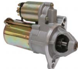
111848 Starter 12 V, 1.0 kW Replacing: D6RA92 Servicing: Chevrolet, Citroen, Daewoo, Holden, Isuzu, Opel, Peugeot, Vauxhall B+ M8, Total length 215.50, Gear type GR, Mounting holes 2 (1) A: 82.50 B: 19.00 mm
