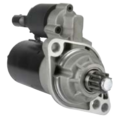
114175 Starter 12 V, 1.1 kW Replacing: 0001121411, 0001121410, 0001120411, 0001120410 Servicing: Audi, Seat, Skoda, VW B+ M8, Total length 223.00, Gear type GR, Mounting holes 3 (0) A: 76.00 B: 56.00 mm
