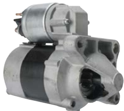
113932 Starter 12 V, 0.85 kW Replacing: TS10E3, D7E47, D7E27 Servicing: Dacia, Nissan, Renault B+ M8x1.25, Total length 168.00, Gear type DD, Mounting holes 3 (3) B: -3.00 mm
