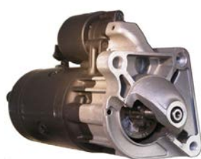
111905# Starter 12 V, 2.2 kW Replacing: D7R23 Servicing: Renault B+ M8, Total length 237.00, Gear type GR, Mounting holes 3 (2) A: 71.50 B: -7.00 mm
