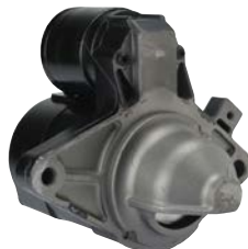
113963 Starter 12 V, 1.1 kW Replacing: TS10E1 Servicing: Citroen, Peugeot, Toyota B+ M8, Total length 168.40, Gear type DD/GR, Mounting holes 2 (1) A: 74.00 B: 25.00 mm
