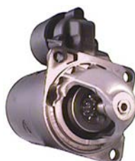
110336 Starter 12 V, 0.75 kW Replacing: D9E167, D9E107 Servicing: Ford, Mercury, Triumph B+ M8, 15a M5, Total length 224.50, Gear type DD, Mounting holes 3 (0) A: 89.00 B: 28.00 mm
