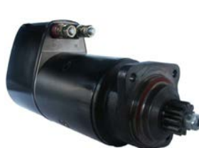
110209 Starter 24 V, 5.4 kW Replacing: 9125420 Servicing: DAF B+ M12, B- M12, Total length 387.00, Gear type DD, Mounting holes 3 (0) A: 89.00 B: 47.00 mm
