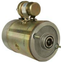
112527 # DC Motor 24 V, 2.5 kW Replacing: AMJ5707, 11.216.133, 19024696, 19024694 OD 114.50, Total length 205.00, Pulley w/o, Rpm./ max. 2100
