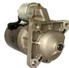
112541 Starter 12 V, 2.2 kW Replacing: D11E272, D11E172 Servicing: Fiat, Jeep, Renault B+ M8, Total length 273.00, Gear type DD/GR, Mounting holes 2 (1) A: 77.00 B: -4.00 mm
