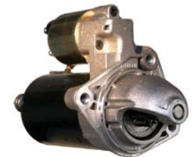
111906 Starter 12 V, 1.1 kW Replacing: TS12E10 Servicing: Ford, Mazda, Volvo B+ M8, Total length 214.35, Gear type GR, Mounting holes 3 (3) A: 76.00 B: 26.35 mm
