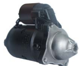
111068 Starter 12 V, 0.85 kW Replacing: 534048 Servicing: Citroen, Peugeot, Talbot B+ M8, Total length 212.25, Gear type DD, Mounting holes 3 (3) A: 65.85 B: 15.65 mm
