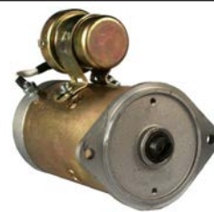
112520 # DC Motor 12 V, 0.8 kW Replacing: 19024676 OD 78.50, Total length 175.00, Rpm./ max. 2700
