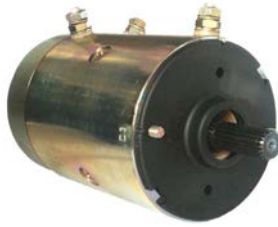
112574 DC Motor 12 V, 1.6 kW Replacing: AMJ4761, AMJ4635, 11.216.273 OD 112.00, Total length 230.00, Pulley w/o, Rpm./ max. 2800
