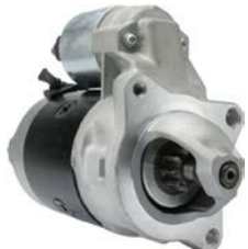
110866 Starter 12 V, 0.9 kW Replacing: 534047, 534032 Servicing: Renault B+ M8, Total length 197.65, Gear type DD, Mounting holes 3 (2) A: 66.00 B: 10.50 mm
