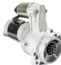
113937 Starter 12 V, 2.2 kW Replacing: TM000A23601, 1250128 Servicing: Hyundai, Kia B+ M8, Total length 240.00, Gear type GR, Mounting holes 2 (2) A: 78.00 B: 16.50 mm
