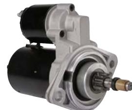
110363 Starter 12 V, 0.7 kW Replacing: D8E158 Servicing: BMW, Porsche, VW B+ M8, Total length 214.00, Gear type DD, Mounting holes 2 (0) Bushing D.E. (clutch house): Cargo 140008. A: 76.00 B: 33.00 mm
