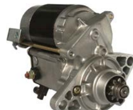
113024 Starter 12 V, 1.6 kW Replacing: D7RSA9, D7RSA3 Servicing: Honda B+ M8, Total length 211.00, Gear type GR, Mounting holes 2 (0) A: 75.00 B: 33.00 mm
