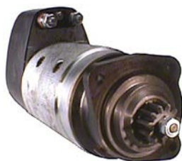
110205 Starter 24 V, 6.5 kW Replacing: 9125100 Servicing: Volvo B+ M12, Total length 407.00, Gear type DD, Mounting holes 3 (0), Waterproof A: 89.00 B: 47.50 mm
