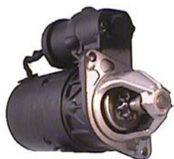
110856 Starter 12 V, 0.6 kW Replacing: 6219, 6185, 6136, 532023, 532021 Servicing: Renault B+ M8, Total length 208.50, Gear type DD, Mounting holes 2 (0) A: 66.00 B: 21.00 mm
