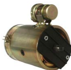
112512 # DC Motor 24 V, 3 kW Replacing: 19024657 OD 114.50, Total length 199.00, Pulley w/o, Rpm./ max. 4800
