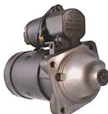
110338 Starter 12 V, 0.8 kW Replacing: D9E127 Servicing: Fiat, Lancia, Zastava B+ M8, Total length 254.00, Gear type DD, Mounting holes 3 (3) A: 66.90 B: 12.00 mm
