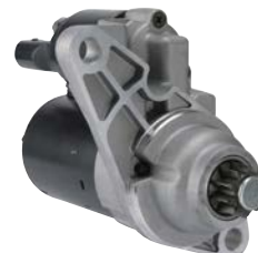
114034 Starter 12 V, 1.0 kW Replacing: TS10E26, D6GS12 Servicing: Audi, Seat, Skoda, VW B+ M8, Total length 194.00, Gear type GR, Mounting holes 2 (0) A: 76.00 B: 52.50 mm
