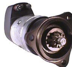
110213 Starter 24 V, 6.6 kW Replacing: 9125020 Servicing: Fiat, Iveco B+ M12, B- M10, Total length 407.00, Gear type DD, Mounting holes 3 (0) A: 115.00 B: 20.80 mm
