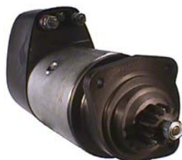
110207 Starter 24 V, 5.4 kW Replacing: 9125240 Servicing: Volvo, Volvo BM B+ M10, B- M10, Total length 387.00, Gear type DD, Mounting holes 3 (0) A: 89.00 B: 47.00 mm
