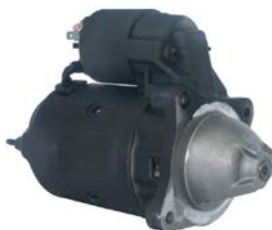
111064 Starter 12 V, 1.05 kW Replacing: 534044, 534023 Servicing: Renault, Volvo B+ M8, Total length 207.00, Gear type DD, Mounting holes 3 (3) A: 65.90 B: 11.00 mm
