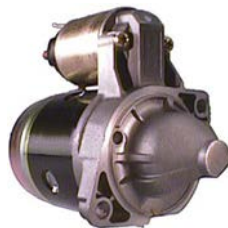
110315 Starter 12 V, 0.9 kW Replacing: MC109025, MC109018, M39646, M37454, M36370, 1EM0081 Servicing: Dodge, Hyundai, Kia, Mitsubishi, Plymouth, Proton B+ M8, Total length 188.93, Gear type DD, Mounting holes 2 (2) A: 76.00 B: 18.40 mm
