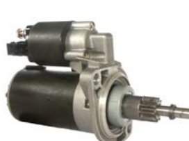
111749 Starter 12 V, 1.1 kW Replacing: 66925322, 66925263, 35258640 Servicing: Audi, Ford, Seat, Skoda, VW B+ M8, Total length 245.00, Gear type GR, Mounting holes 2 (0) Bushing D.E. (clutch house): Cargo 140018. A: 76.00 B: 52.00 mm
