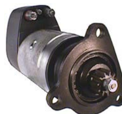
110214 Starter 24 V, 6.6 kW Replacing: 9125120 Servicing: Scania B+ M12, B- M12, Total length 407.00, Gear type DD, Mounting holes 3 (0), Insulated return A: 92.00 B: 37.00 mm
