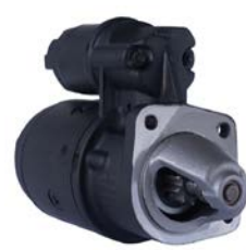
111104 Starter 12 V, 0.9 kW Replacing: 534002 Servicing: Alfa Romeo B+ M8, Total length 229.00, Gear type GR, Mounting holes 3 (0) A: 61.90 B: 10.00 mm
