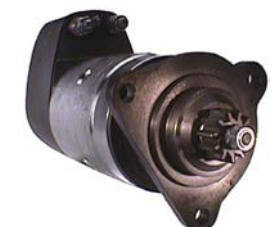
110211# Starter 24 V, 6.6 kW Replacing: 9125140 Servicing: Scania B+ M12, B- M12, Total length 407.00, Gear type DD, Mounting holes 3 (0), Insulated return A: 92.00 B: 48.00 mm
