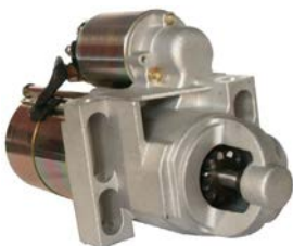
110216 Starter 12 V, 1.4 kW Replacing: A16R261T Servicing: Buick, Cadillac, Chevrolet, GMC, Mercedes, Oldsmobile, OMC, Pontiac B+ M8, Total length 236.00, Gear type DD, Mounting holes 2 (0) Replacing: 10MT. A: 68.00 B: 0.00 mm
