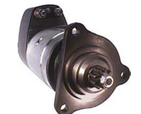
110210 Starter 24 V, 6.6 kW Replacing: 9125010 Servicing: Fiat-Allis, Kässbohrer, MAN, Mercedes-Benz, Mitsubishi, Neoplan, Ssangyong B+ M12, B- M10, Total length 407.00, Gear type DD, Mounting holes 3 (0) A: 92.00 B: 48.50 mm
