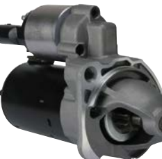
114179 Starter 12 V, 1.2 kW Replacing: 0001107428, 0001107427 Servicing: Audi, Seat, Skoda, VW B+ M8, Total length 200.00, Gear type GR, Mounting holes 2 (2) A: 82.50 B: 15.45 mm
