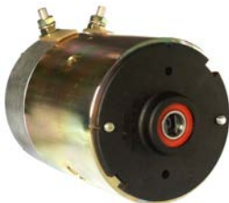
112573 DC Motor 12 V, 1.6 kW Replacing: AMJ5705, AMJ5666, AMJ5175, 11.216.117, 11.212.609, 11.212.107 OD 114.50, Total length 173.00, Pulley w/o, Rpm./ max. 2600
