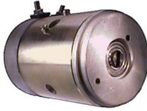
111091 DC Motor 24 V, 2.5 kW Replacing: 0136355081, AMJ5592, 11.212.417, 19024678 OD 117.00, Total length 195.60, Pulley w/o, Rpm./ max. 2100
