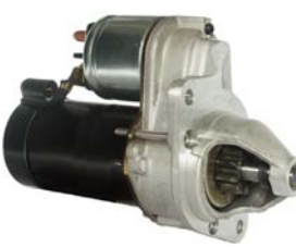
111100 Starter 12 V, 0.7 kW Replacing: 6202F, 6202D, 6202C, 6202B, 6202A, 6202 Servicing: Citroen B+ M8, Total length 207.75, Gear type DD, Mounting holes 2 (0) A: 65.60 B: 19.80 mm
