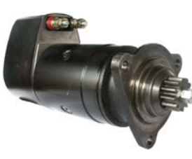
111983# Starter 24 V, 6.6 kW Replacing: 860517 Servicing: Mercedes-Benz, Volvo B+ M10, B- M10, Total length 406.00, Gear type DD, Mounting holes 3 (0), Insulated return A: 92.00 B: 47.00 mm
