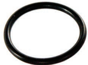
252596 # O-ring ID 24.00, Thickness 2.50, Material Rubber
