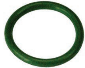
250495 O-ring Servicing: Opel, Vauxhall ID 14.81, Thickness 1.88, Material HNBR
