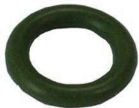
250454 O-ring Replacing: 92471-N8210 Servicing: Alfa Romeo, Fiat, Ford ID 6.80, Thickness 1.87, Material HNBR
