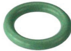
251013 O-ring ID 6.50, Thickness 1.50, Material HNBR
