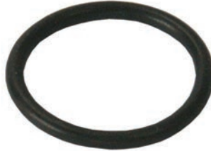
251289 O-ring Servicing: 02131-9110, 02131-9111 ID 18.00, Thickness 2.00, Material Nioprene
