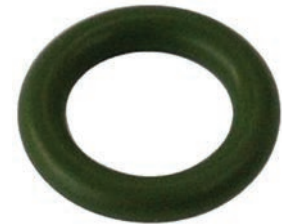
250462 O-ring Servicing: BMW, Ford, Opel, Vauxhall ID 9.19, Thickness 2.62, Material HNBR
