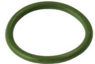
250499 O-ring ID 21.60, Thickness 2.40, Material HNBR
