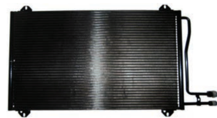
260078 Condenser Replacing: A9015000554, A9015000454, 9015000554, 9015000454 Servicing: Mercedes-Benz Dryer w/o A: 380.00 B: 670.00 C: 21.00 mm
