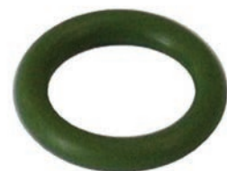
250465 O-ring Servicing: Ford, Mazda, Opel, Vauxhall ID 7.38, Thickness 1.81, Material HNBR
