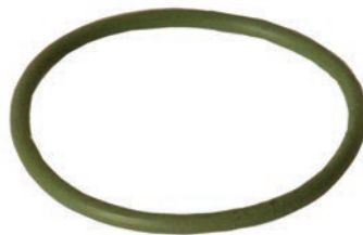
251424 O-ring ID 28.30, Thickness 1.78, Material Nioprene
