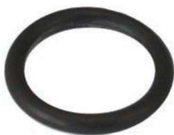
250476 O-ring Servicing: Suzuki, Toyota ID 15.00, Thickness 2.50, Material Nioprene
