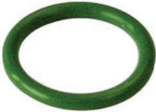
250501 O-ring ID 12.42, Thickness 1.78, Material HNBR
