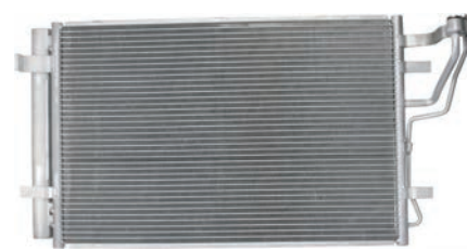
260406 Condenser Replacing: 976061H000 Servicing: Kia Dryer w/ A: 391.00 B: 608.00 C: 20.00 mm
