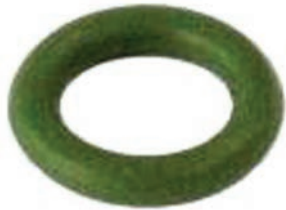
250484 O-ring Servicing: Honda, Acura, Nissan, Calsonic, Renault ID 4.70, Thickness 1.42, Material HNBR
