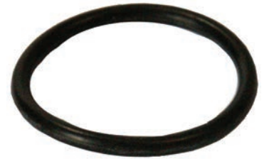
251425 O-ring ID 26.65, Thickness 2.62, Material Nioprene
