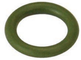
250463 O-ring Servicing: BMW, Honda, Acura, Mitsubishi, Nissan, Calsonic, Opel, Vauxhall ID 10.77, Thickness 2.62, Material HNBR
