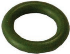
250452 O-ring Servicing: Alfa Romeo, Ford, Mitsubishi, Nissan, Calsonic, Renault ID 6.07, Thickness 1.78, Material HNBR
